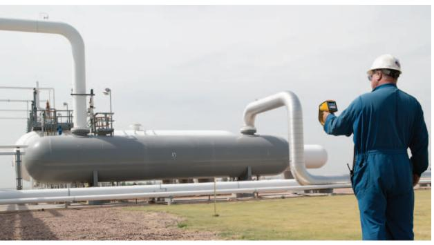
Thermal images of this sludge catcher vessel revealed the line between unrefined natural gas and heated sludge, saving the plant from a major shutdown required for manual verification.
